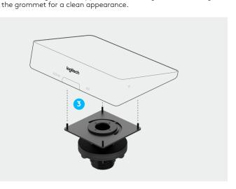
Cable Management: Supports down-routing of cables through
